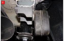
F) Both of the rear mounting points need rotating 180° when fitting the Scorpion exhaust.
